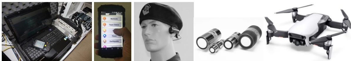
Figure 3: Examples of PPDR ONE user terminal and IoT devices – ruggedized industrial platforms, ruggedized Android terminal, wearable cameras, water sensors, drone.
